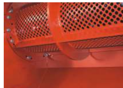
The screen size perforation determines the chips size
