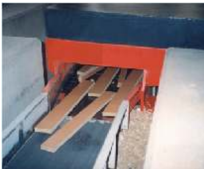
LEOPARD in a pit connected directly to a panel dividing saw
